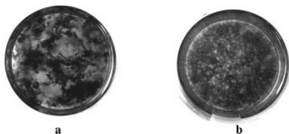
Figure 7 The appearance of the hydrogels after adsorption of basic dye. (a) S-g-AA/MMT-1 , (b) S-g-AA/MMT-0 .
